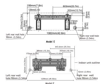
**NOTE:** When the gas side connective pipe is  $\Phi$  16mm(5/8in) or more, the wall hole should be 90mm(3.54in).
