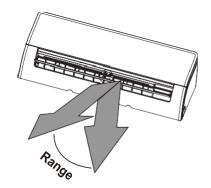
**NOTE:** Do not move louver by hand. This will cause the louver to become out of sync. If this occurs, turn off the unit and unplug it for a few seconds, then restart the unit. This will reset the louver.
