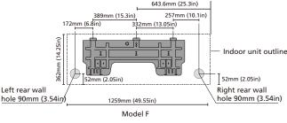
**NOTE:** When the gas side connective pipe is  $\Phi$  16mm(5/8in) or more, the wall hole should be 90mm(3.54in).
