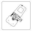
Remove batteries from remote control
